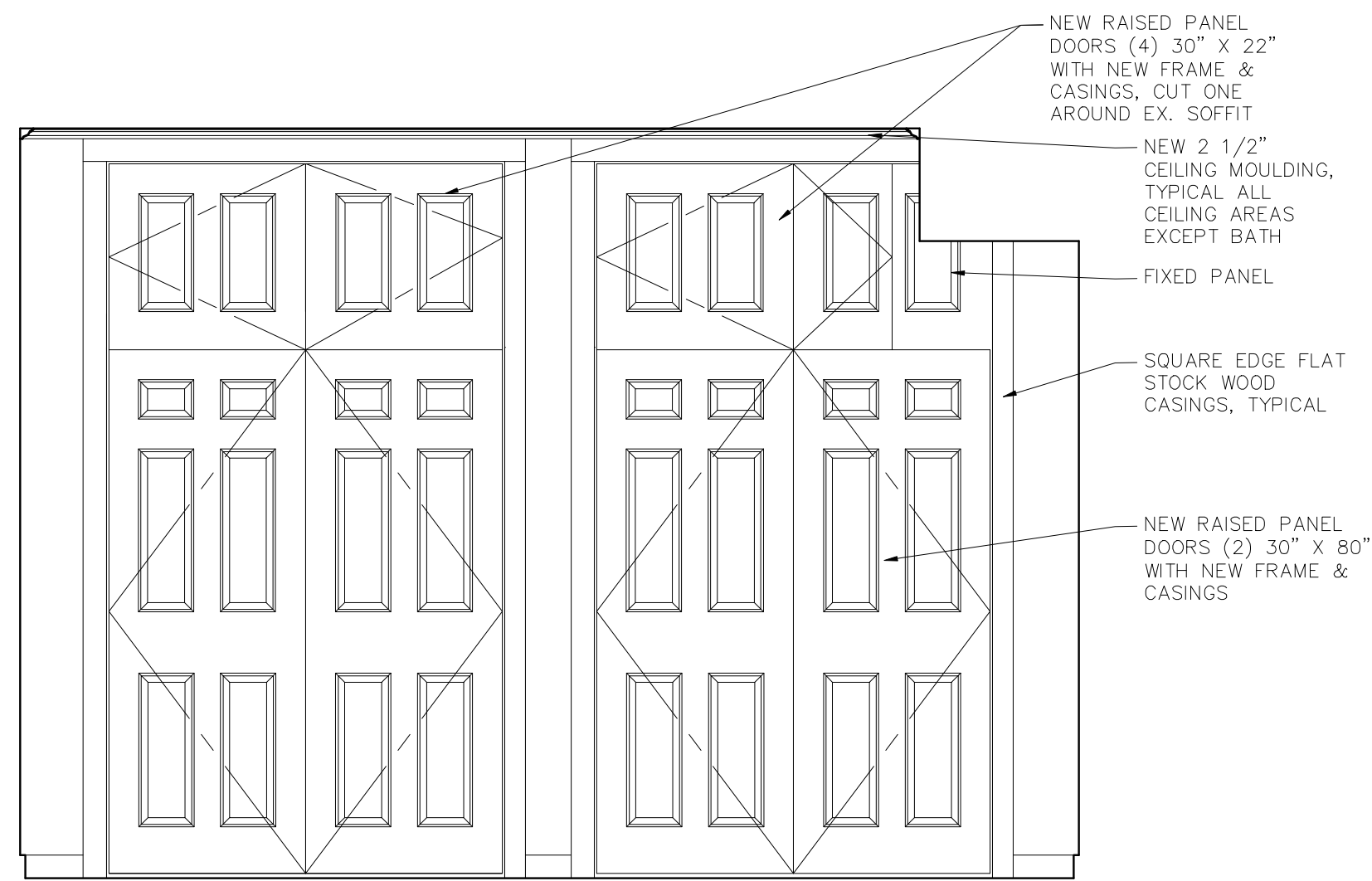
1 GREEN ROOM CLOSET DOOR ELEVATIONS A401 SCALE: 1/2" = 1'-0"
