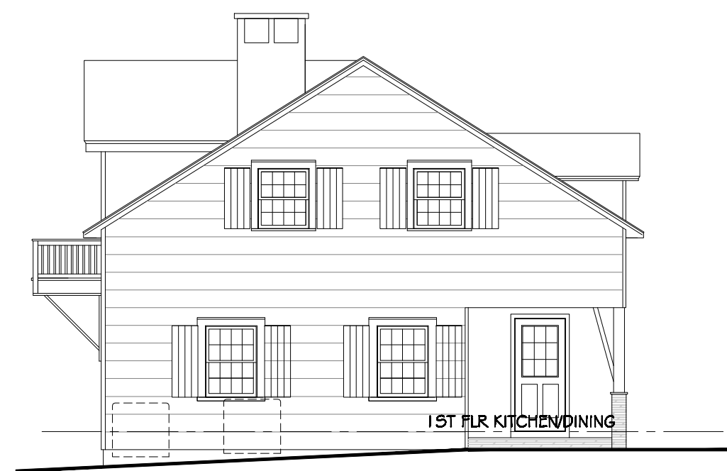
3 A200 EXISTING SIDE ELEVATION - NORTH SCALE: 1/8" = 1'-0"
